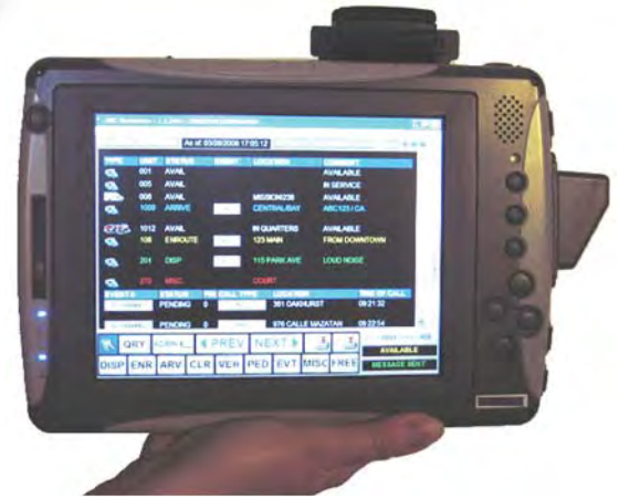
MDC Workstation shown running on a Touch-Screen tablet with a broadband card and built-in GPS. -- Totally Portable! --
